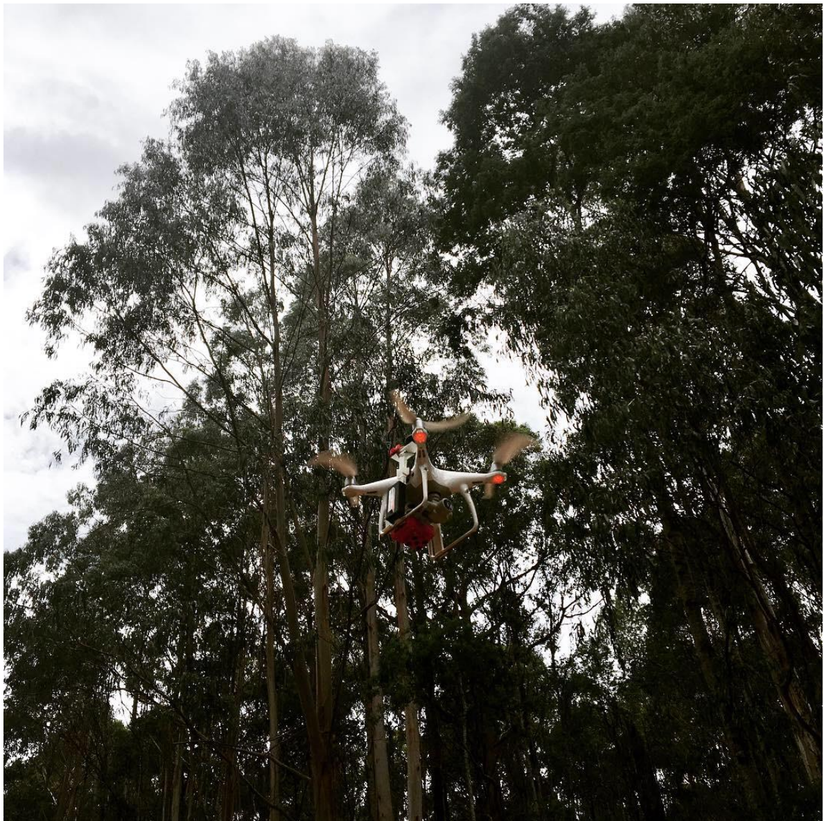
Figure 4. Our multirotor UAV, modified to carry a multispectral camera, lifting off to capture imagery of one of our study sites near Mount Jersey
