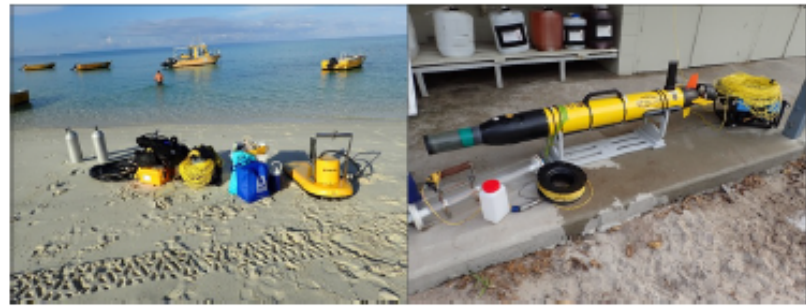
A SEA OF YELLOW: PREPARING THE SURVEY EQUIPMENT FOR FIELDWORK AT LIZARD ISLAND RESEARCH STATION; EDGETECH SUB-BOTTOM PROFILER (LEFT) AND IVER ECOMAPPER AND BLUEROV2 (RIGHT). © MARDI MCNEIL
